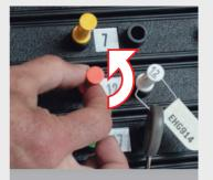
By turning the access peg, the system is activated and the desired key is released.
