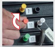
The colored access peg is inserted to remove the desired key from the system.
