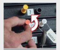
By turning the access peg, the system is activated and the desired key is released.
